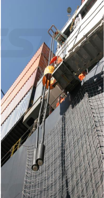
Cable management system on board container vessel
