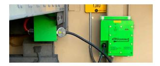
Unlike competing technologies, ESL's innovative design does not require 2 extra pilot pins at the connector. A connection detection device is embedded in the safety-interlocked IEC female plug installed at the end of the cable. This allows truck owners to use the OEM provided inlet for plug-at-front configuration or retrofit their fleet with ESL's cost effective plug-at-rear kit.
